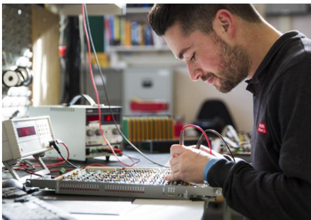
Normally, a functional test only proves that the assembly basically operates. It does not usually detect the presence of faults in parts used as protection elements, which are inactive under normal operating conditions. Furthermore an assembly failing functional test will often need very skilled analysis to identify and rectify the root cause of failure.
